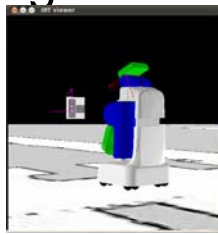
Pr2 kinematic model for push-button motion and visually detected panel location
